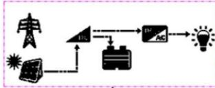
When PV power is lower than or equal to load power, PV stops charging the battery, and it supplies the load together with the battery.
