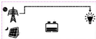
The battery voltage goes lower than or equal to AON. Simultaneously, it has not been charged to AOF. The utility supplies the load and charges the battery.
