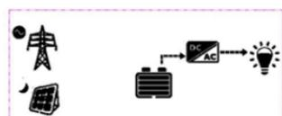
When the battery voltage goes lower than or equal to the LVD point, utility supplies the load.
