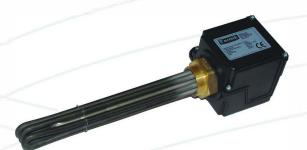
Immersion Heater with integrated Isolation for direct water heating, especially useful in enameled tank. It consists of three "U" shaped tubular heating element and a sensor protection tube mounted in a screw head G 1 1/2". The Heater is with a plastic housing, in which a temperature control (30-75°) with a limiter (98°C) and indicator lamp is provided. The isolated construction of the tubular heater protects enamelled tank against corrosion.
